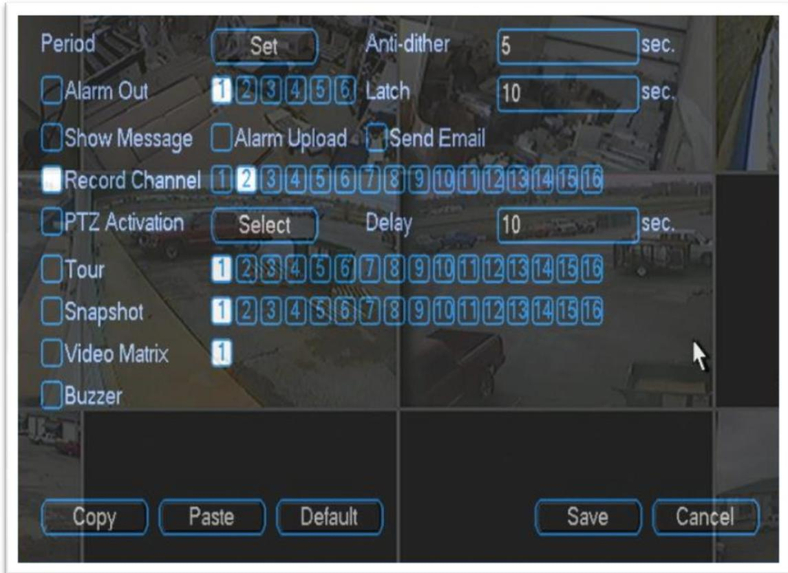
**Step 4.** Now that we have our Alarm setup correctly we need to set the alarm to **Schedule** on our DVR. To do so, access the **Schedule** screen under the options menu.
