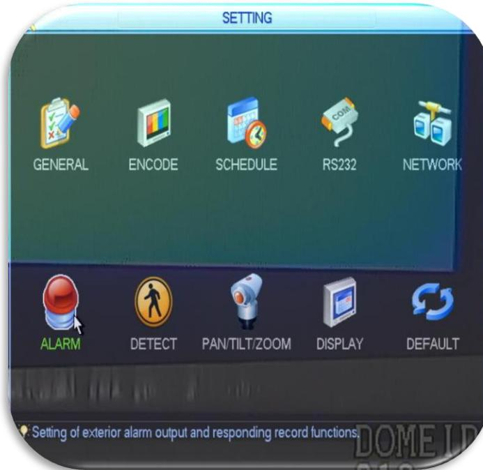
**Step 3:** Now that we are inside the Alarm settings window we will need to concentrate on a few areas to setup our PTZ preset with our Alarm. First make sure you have your proper alarm device input selected in “Alarm In”, Next, under Record Channel it will say PTZ Activation and have a blank box next to it. Click that box to **enable** your PTZ activation. Once this is complete click the **Select** button next the words PTZ Activation to bring up the Preset window.
