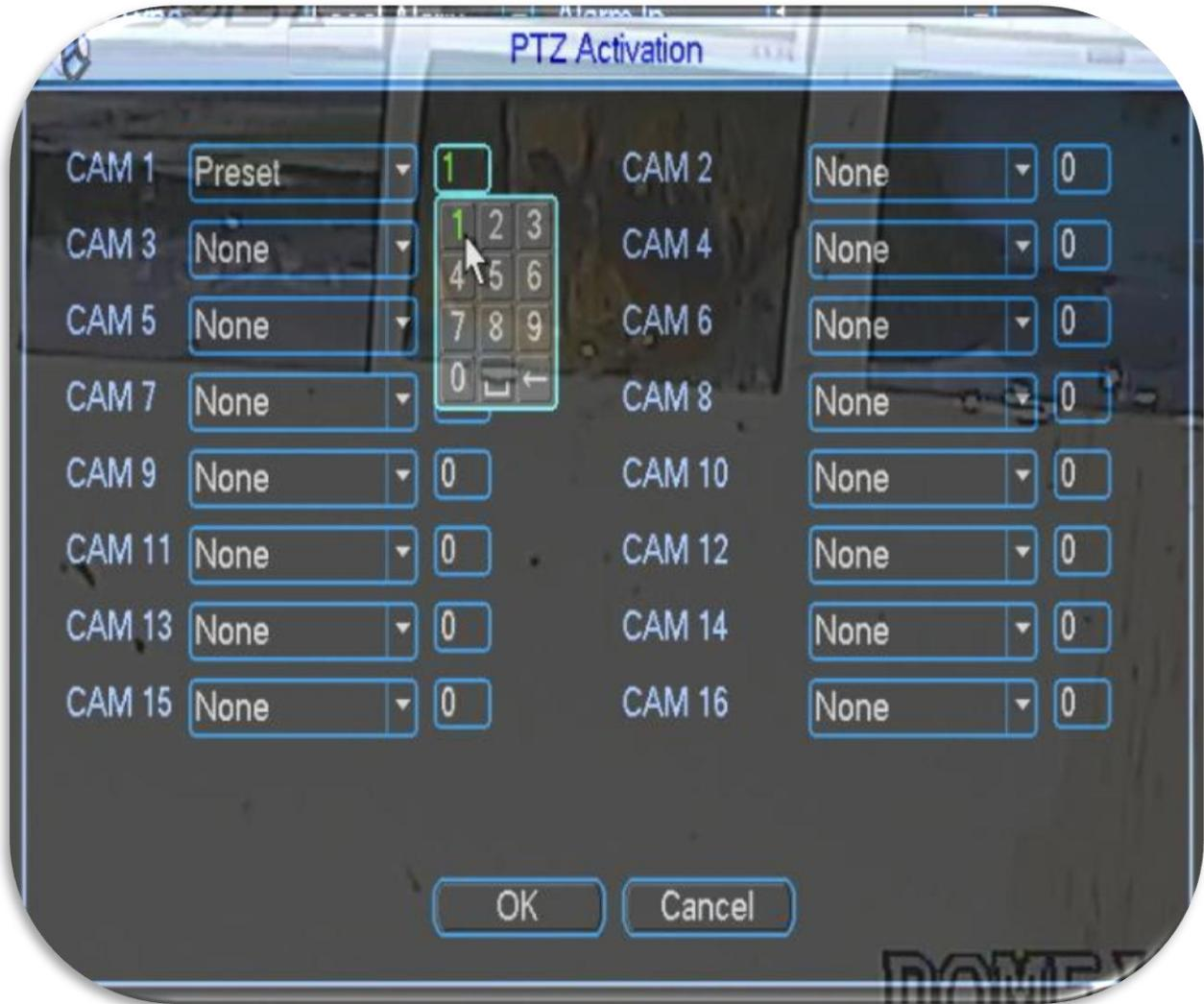
**Step 5:** Once you have clicked **OK** and are viewing your PTZ's view, test out your work by activating your Alarm Device and watch your preset in action.
