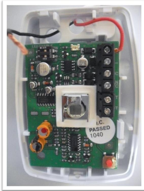
**Step 3:** Next, we will need to **connect the negative power wire** to the negative port on our PIR sensor.
