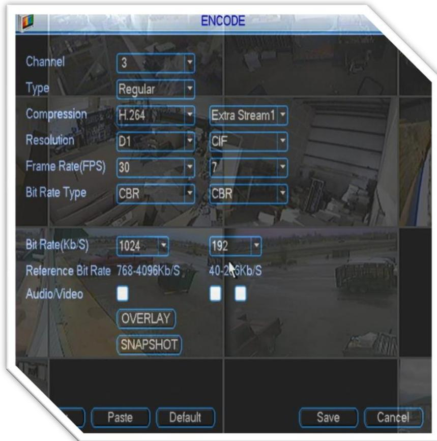
**Step 4:** If you haven't already connected a microphone to your audio input for your selected camera channel now, is a good time. Simply connect the microphones cable to the **Audio In port for your channel**. For example, we want to record on channel 3 therefore our microphone will be connected to the **Channel 3 Audio In port on the back of our DVR**. Also your microphone will need a **power source**, connect that to power the mic.
