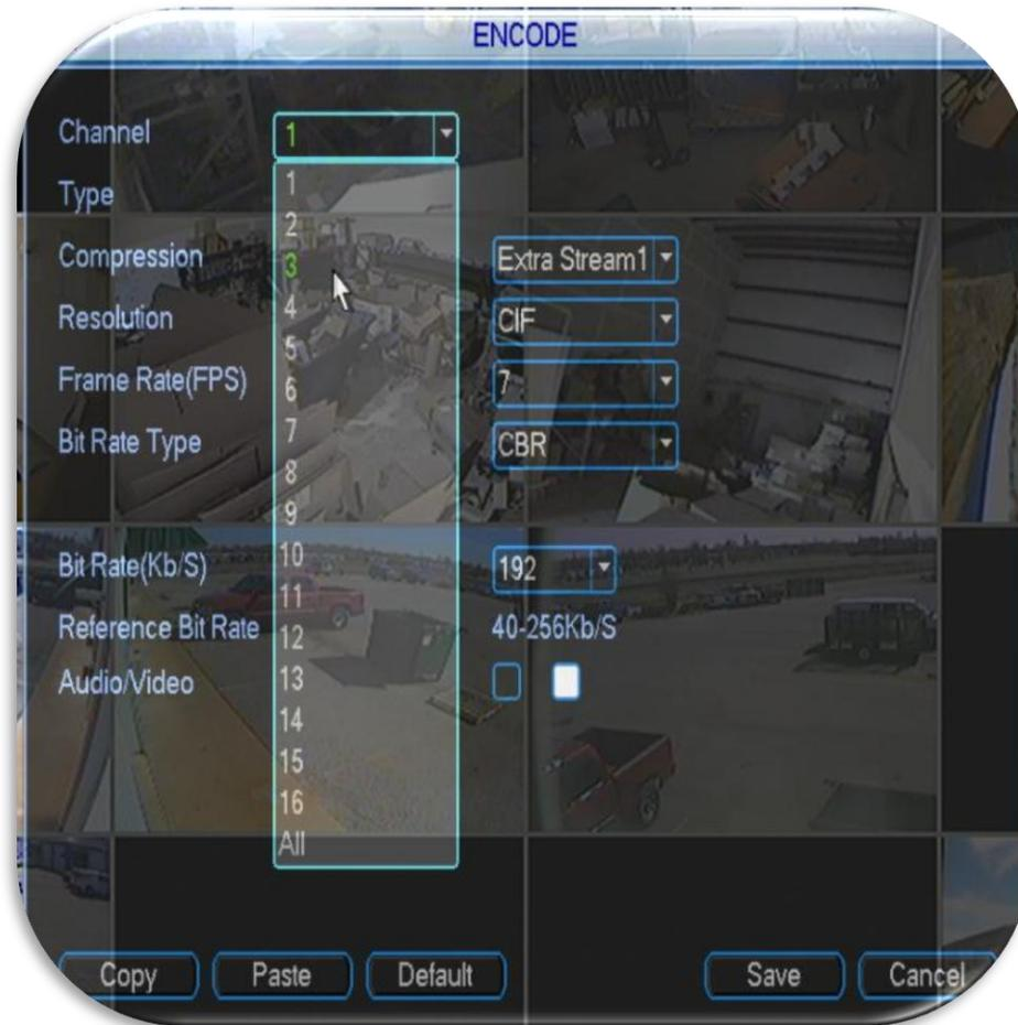
**Step 3:** Now that we have our correct channel selected let's activate audio recording by **clicking in the box** next to **Audio/Video** to fill it in, also the box directly to the right of the box you just filled in will activate audio for the **ExtraStream** option, **click** it to activate audio on ExtraStream also. Once this is done click the **Save** button at the bottom.
