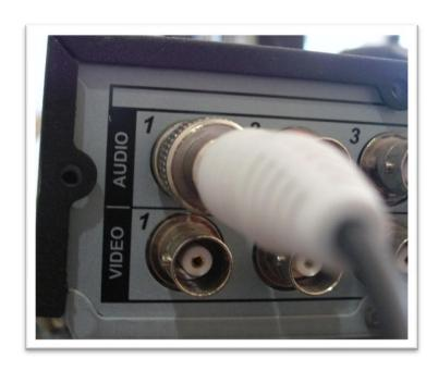
**Step 2:** Now that we have a microphone connected to the DVR we will need to connect a cable from the **Audio Out**on the DVR to an **Audio Input** on the TV/Monitor or to external speakers.
