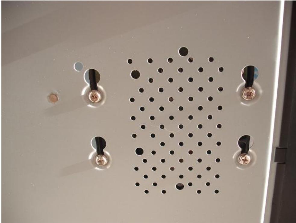
**Step 6:** Replace the cover to the DVR and screw it back into place.
