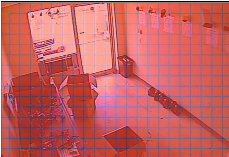
Now say for example that I wanted the door in this picture to not be subject to motion detection triggers. To do this, I would simply click on the boxes around the area of the door. Or I can simply click and drag my mouse cursor to the area selection that I want to be blocked for motion detection. The following picture shows what this will look like. So if anyone walks into the area that has the clear “non-
