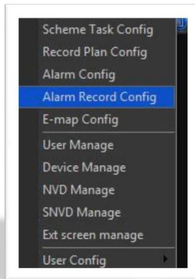
**Step 2:** Now that we are viewing the Alarm Record Config window you will notice your **device name** in the left column. Click the **[+] arrow** next to the device to expand the list with your camera names. Next we need to select which camera we would like to setup for Motion Detection Alarm Recording. For our example we will begin with **CAM 6**, go ahead and click your cam name now to **highlight it**.
