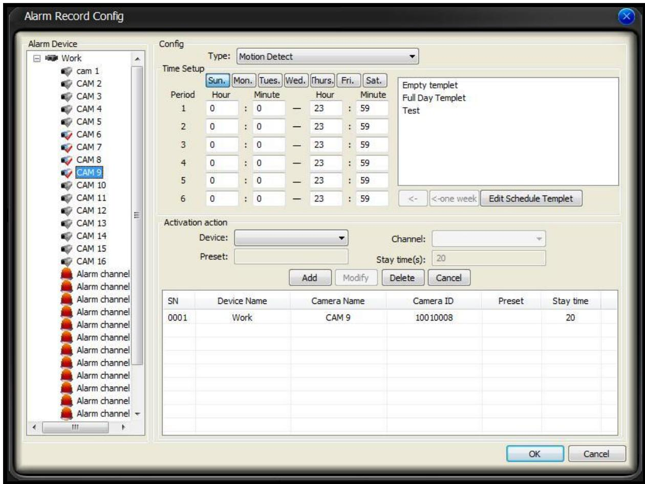
**Step 5:** Now that we have our cameras setup and the **Alarm Arm Enabled** we can check our folder for recordings whenever motion was detected. Once you have created motion to test the configuration browse to the default download folder for PSS recordings: **C:\PSS Downloads**. Inside this folder should be one or two more folders, one labeled with the date of the video capture, inside that should be your recordings.
